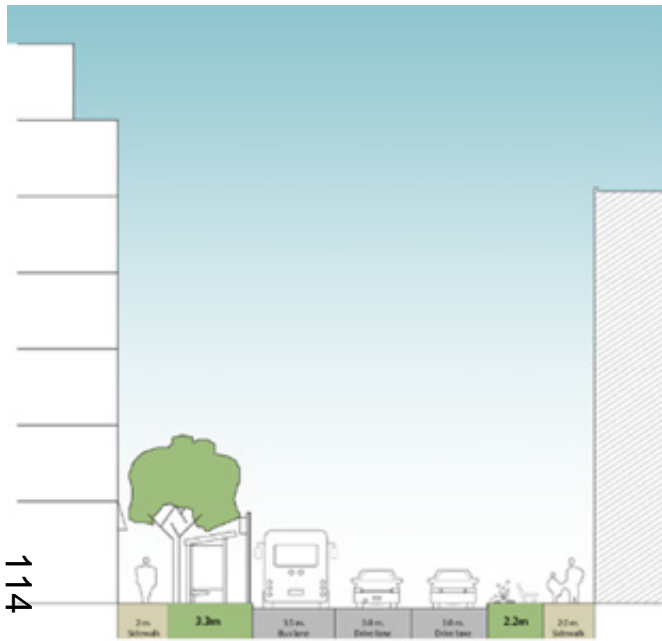
Figure 8.31: Section through Station Road
